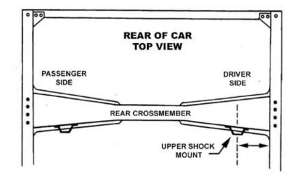
LOCATE UPPER SHOCK MOUNT ABOUT 9" TO 10" FROM THE INSIDE OF THE FRAME RAIL TO THE CENTER BOLT
