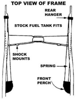
\*TIP: TO DETERMINE THE ANGLE OF THE REAR HANGER, FIRST INSTALL FRONT PERCH AND TEMPORARILY BOLT IN SPRING WITH SHACKLE IN PLACE.
